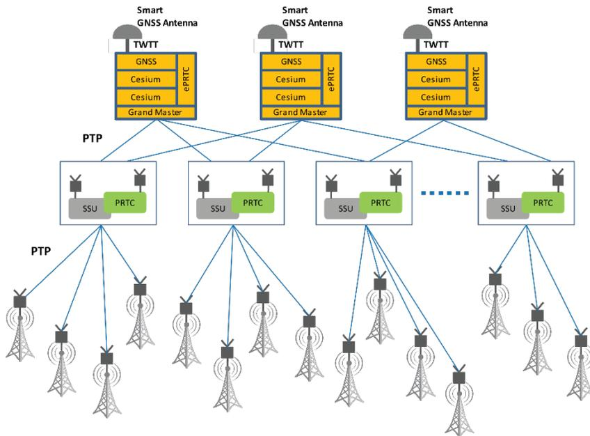
The architecture in the previous illustration limits the core and aggregation synchronization network to just two layers: the Leaf (Aggregation nodes) and Spine (Core nodes). This helps to maintain predictability between the ePRTC and subtending SSU and PRTC systems.
