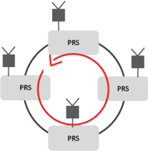
Over the last decade, distributed PRS has become a pervasive solution for timing in network cores, to the point where hundreds, and in some cases thousands, of GNSS receivers are relied upon for network synchronization.
