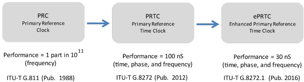
The remainder of this paper looks at the components that comprise an ePRTC system, and how this system performs in both normal operating conditions and during GNSS outages.
