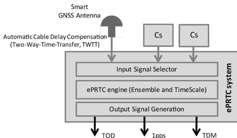
Inputs to the ePRTC system include an interface for the smart GNSS antenna along with 10 MHz interfaces to external atomic clocks (typically cesium). At a minimum, a GNSS input and at least one cesium clock should be connected.
