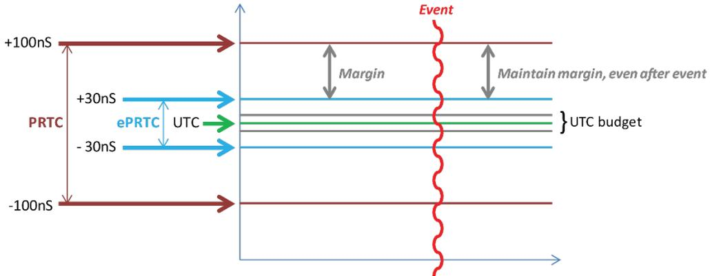
The diagram above provides a simple view of the performance objectives for the ePRTC. It is important to note that the 30 nS accuracy should be maintained during normal operating conditions (when GNSS is available) and, even more importantly, after an event such as when a GNSS outage has occurred.
