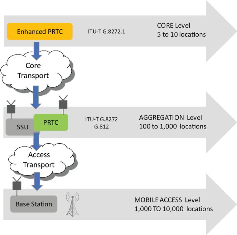
The number of ePRTC locations varies depending on an operator’s network geographical coverage. The key objective is to deliver the highly-accurate time produced by the ePRTC to each aggregation node with minimal time error and with the highest possible level of efficiency, scalability, and fault tolerance.
