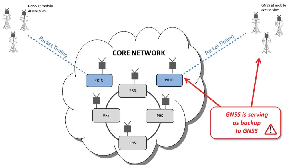
Although the deployment of PRTC systems in the core network to deliver frequency and time over packet networks to mobile access points has proven to be a viable backup architecture for localized GNSS failures, the ultimate dependency on GNSS in the core network remains. In fact, the GNSS deployed at the mobile access site is actually being backed up by GNSS in the core, and the net result is that the dependency on GNSS remains.
