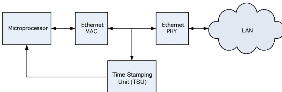
**Figure 2** Hardware set up for a system deploying IEEE 1588. The time stamp unit monitors packets at the MII layer, between the Ethernet MAC and PHY, and issues a precise time stamp when a 1588 timing packet passes through it.
