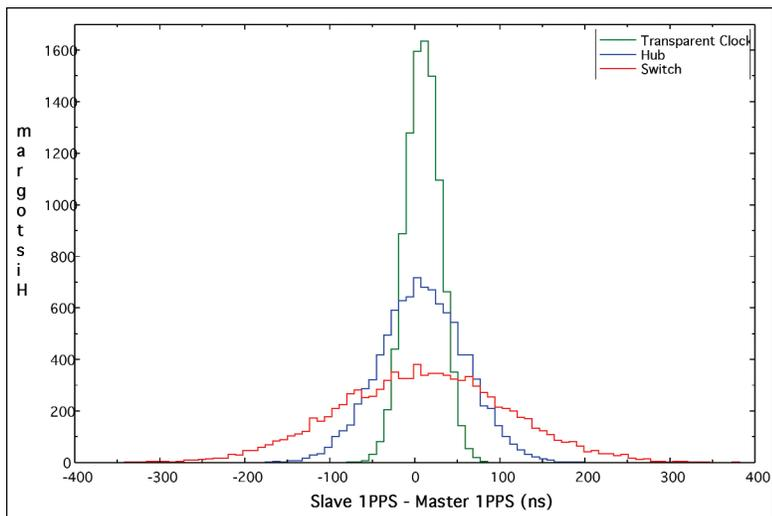
Figure 4 Histograms showing the precision of time synchronization between IEEE 1588 master and slave using three different kinds of Ethernet connection devices.
